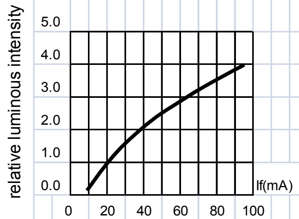
Fig.3 RELATIVE LUMINOUS INTENSITY VS. FORWARD CURRENT.
